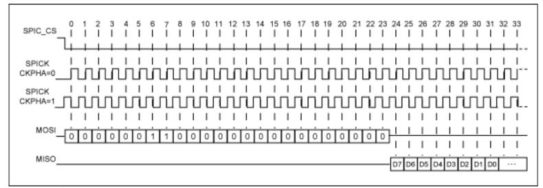
Figure 1. SPI Master Functional Timing
